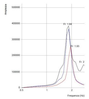
Fig. 2. Increase in frequencies and reduction in amplitudes experimentally recorded. Situation preintervention (blue and black lines) and consolidated situation (red line)
