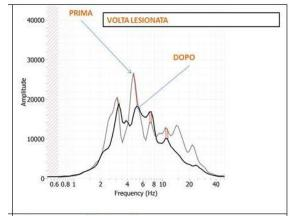
Fig. 5. Experimental frequencies pre and post consolidation intervention on the vaults
