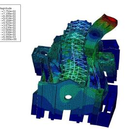
Fig. 4. The numerical FE model of the Cathedral
