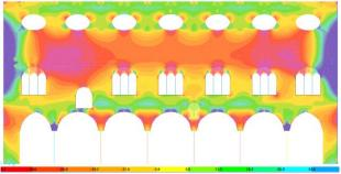
Fig. 7. Numerical state of stress of the Palace, obtained through the calibrated model.
