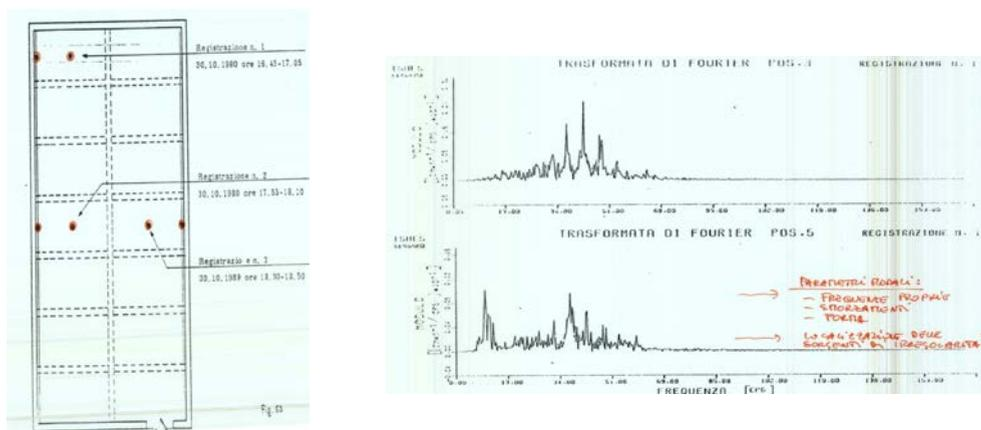
Fig. 2. Dynamic tests recorded on Palazzo della Ragione (1980). Plan view with the position of the accelerometers and accelerogram of two points after application of the Fast Fourier Transform (FFT)
