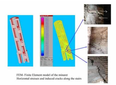
Numerical analyses have highlighted, also here, a marked torsion affecting this minaret. On the basis of the currently data available, we have noted a fairly good correspondence between the pattern of cracks visible on the monument and the areas subject to the greatest stress according to the
